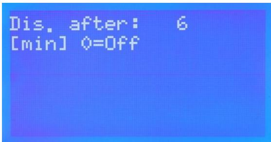
Max. inactive is similar to Stepper inactive but turns everything off. Hot End, Hot Bed, PLA Fans etc. but the lights and main cooling fans stay on.
