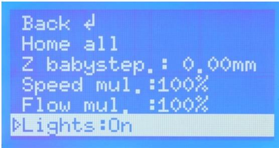
By selecting the Lights option the internal Machine Lighting can be turned on....
