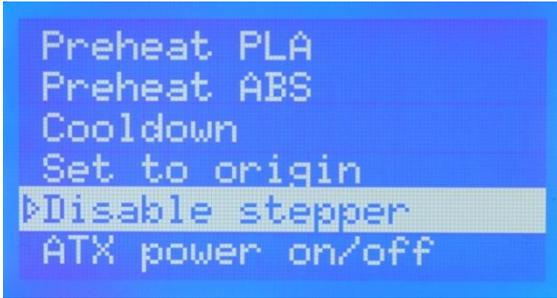
Selecting Disable stepper de-energises (unlocks) all the stepper motors (X,Y and Z) allowing for manual machine mechanism movement. This is particularly useful when manually levelling the printers Hot Bed.
