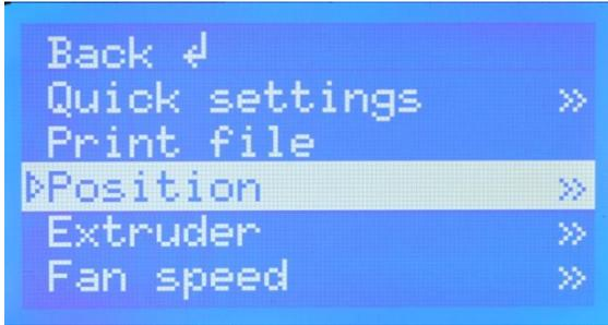
The Position option relates to the position of the X,Y and Z axis.
