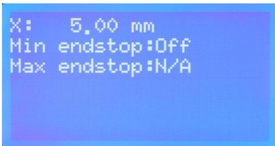
By turning the Jog Wheel the X-axis will move in increments of 1mm.
