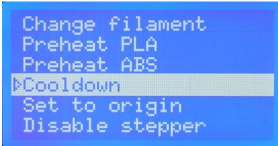
Cooldown can be selected when you require all the heaters (Hot Bed and Hot Ends) to be turned off.
