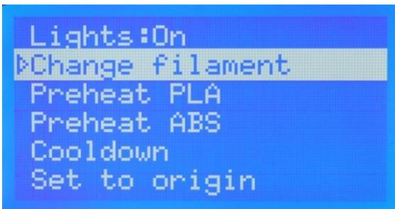
Changing the filament can be done manually or by selecting the Change Filament option shown here.
