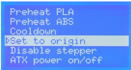
CAUTION. The Hot Ends and Hot Bed will remain hot for several minutes after switching off or after 'Cooldown' is selected
