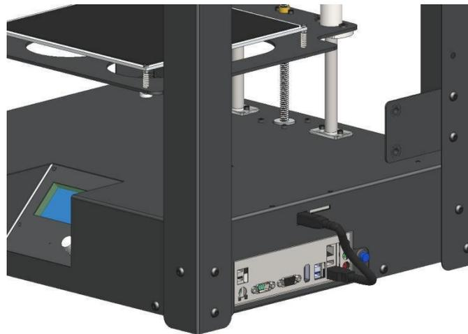
2. Now connect - if PC functionality is required \*\* (ancillary parts not supplied as standard).
